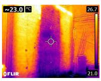
Independent tests have demonstrated that brickwork treated with ProPERLA were significantly more energy efficient than untreated ones. The thermal image shown to the right was taken during independent scientific testing and shows a 6°C difference in temperature between sections of the wall treated with ProPERLA and the untreated centre section.
