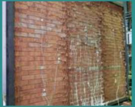
The uncoated bricks (the middle third) showed evidence of water penetration & significant salt effloresence (see image).
