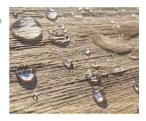
Wooden surfaces which have been treated with ProPERLA Wood Impregnator will respond in the same way, meaning water will form droplets & won't penetrate the timber.
